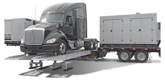
Fig. 2. Render of the mobile chassis dynamometer solution by Taylor Dyno [19]
