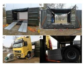
Fig. 7. General view of the mobile dynamometer station: a) front view with ramps; b) back view; c) view with the truck on the dyno; d) view of the wheels of the vehicle on the dyno
