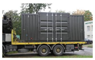
Fig. 8. The diag- dyno station transported on a truck chassis
