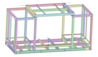
Fig. 4. Technical drawing of the mobile dynamometer support structure
