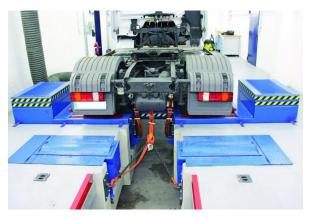
Fig. 1. View of a truck on a chassis dynamometer [16]
